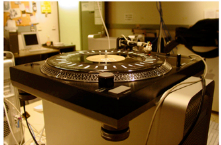
Turntable with optical encoding and accelerometer
